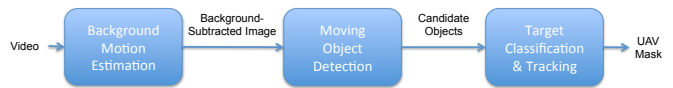
Fig. 2. An overview of our proposed method: We first estimate the background motion between two sequential frames. From resulting background-subtracted image, we detect the moving objects by pruning spurious noise. Among detected objects, we differentiate UAVs from false alarms using spatio-temporal characteristics and track them for temporal consistency.
