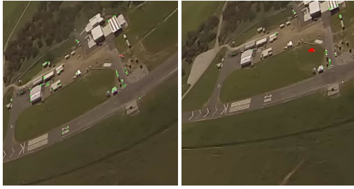
Fig. 4. Shi-Tomasi corner points detected from background subtracted images in two videos: Red and green dots represent pruned and deleted points based on the magnitude of motion difference vector, respectively. We preserve the points around target UAV (red), while deleting the points located at corner of building structures (green). This indicates that the magnitude of difference vector between estimated background and local motion is effective to separate the points in the targets from complex backgrounds. Images are cropped for better display.
