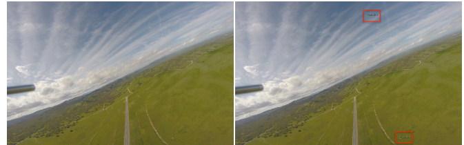
Fig. 1. Challenge in detecting other UAVs: [Left] Original Video, [Right] Video with our detection and tracking; Other UAVs are very small and occluded by complex backgrounds (i.e. cloud) and thus not even recognizable by human eyes. Our proposed method detects and tracks multiple small UAVs successfully as highlighted in red boxes.
